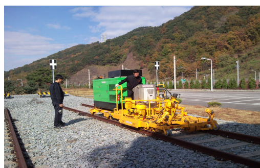
Re-profiling Unit Machine N-320 working in South Korea
