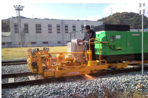
Re-profiling Unit Machine N-320 working in South Korea
